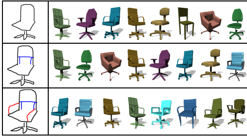
Figure 6: Example of negative (blue) and positive (red) strokes. Top: Initial search results. Middle: Adding negative strokes to suppress the unwanted back support style. Bottom: Adding positive strokes to emphasize the armrests.
